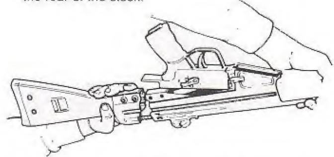
4. The buttstock and driving spring should now remove easily by pulling the butt stock straight back to the rear; the entire buttstock assembly will come out as a unit.
